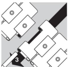
Pull the protruding hinged link out of the bracelet (3). The bracelet is now separated.
