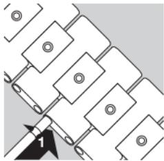
Repeat steps 1 to 3 at the distance from the first point of separation you have just determined. Remove the unnecessary links and reassemble the shortened bracelet. Slide the hinged link into the bracelet sideways (1).
