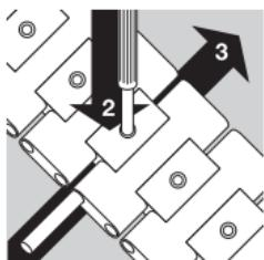
Using the special tool provided, you can now push down the fixing bolt (2) and, at the same time, slide the hinged link back into the bracelet until it lies flush (3). The fixing bolt must be aligned with the upper edge of the securing link. It is important that you check that the hinged link is sitting correctly. Keep the surplus links and separating tool in a safe place for use in any adjustments at another time.
