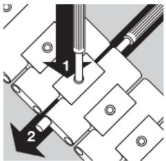
Open the folding clasp by pressing the buttons on the side. Lay the bracelet face down on a firm base. To avoid scratching the bracelet and base, place a cloth underneath the bracelet. Using the special tool provided, you can now push down the fixing bolt at the desired point of separation (1) and, at the same time, slide the hinged link with the help of the second tool about 3 millimetres sideways (2).
