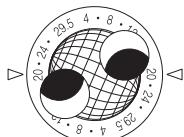
The arrows to the left and right of the moon phase display are used to indicate the days remaining until the next full moon. The period that elapses between one full moon and the next is always exactly 29.530588402 days, which are represented as 29.5 days on the rotating moon phase display, in conjunction with the extremely precise perpetual calendar.
