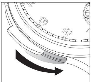
The repeating slide is operated as shown in the illustration. You must always fully depress the slide; otherwise, the repeater will not be activated. This “all-or-nothing” principle ensures that the watch does not chime the time incorrectly. You can then allow the slide to return to its original position.
