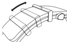
A metal loop (3) is available to secure the loose end of the bracelet in position. This is infinitely adjustable and can be moved effortlessly to the desired position.
