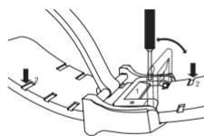
Lay the bracelet with its top surface on a firm base with the clasp fully open. Located beneath the outer side of the clasp is the clamp fastener that holds the bracelet in position. The locking lever on the clamp fastener (1) can be opened simply by inserting the special tool supplied
