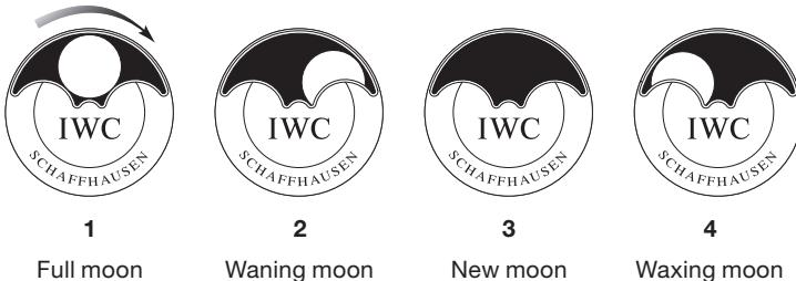
The moon phase display is set automatically by the date-mechanism and is thus always correct. The reduction ratio is so precise that the display will only deviate by a single day after 577 years.
