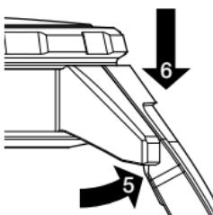
Now return the bracelet or strap to its original position (5) while simultaneously pressing it down into the horns to snap it into place (6).
