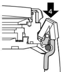
To attach the bracelet or strap, hook the notch of the horns from above into the spring pin of the case (4).
