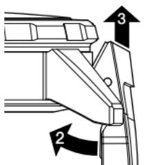
Tilt the bracelet or strap inwards (2) and move it upwards away from the case (3).
